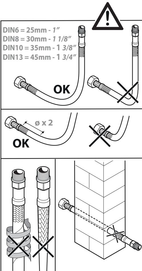
**EN** **INSTALLING THE FLEXIBLE HOSES (SUPPLIED): warning**
