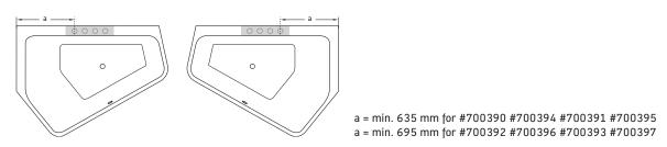
3rd step: Specify the dimensions for drilling the holes. Please enter the distance between them and the diameter for each hole directly in the drawing.
